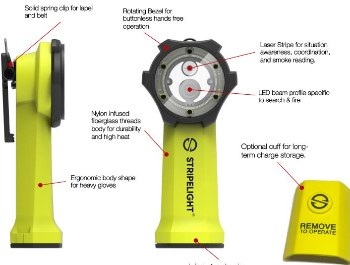
The Stripelight FRT L1 Model is a handheld fire, rescue, and tactical (FRT) intrinsic safe flashlight specific to HazLoc US/Canada certifications. It provides a blue Laser stripe line and LED light sources. The FRT L1 laser provides new functionality for situation awareness to first responders to identify obstacles, holes, or search for others providing hints to navigation and to observe smoke flow, density, and track source.
