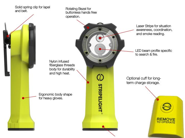
The Stripelight FRT EX Model is a handheld fire, rescue, and tactical (FRT) intrinsic safe flashlight specific to Atex/IECEx certifications. It provides a blue Laser stripe line and LED light sources. The FRT EX provides new functionality for situation awareness to first responders to identify obstacles, holes, or search for others providing hints to navigation and to observe smoke flow, density, and track source. In inductive charging, no electrodes.
